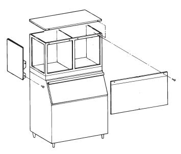
3. Remove two screws at the front of each side panel, and pull them forward until they release from the tabs connecting them to the back panel. Evaporator Cover:
