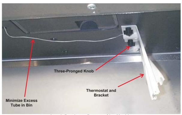
Attach Bracket to Bottom of Ice Machine
