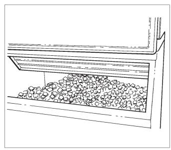
Typical Ice Level When Unit Shuts Off
